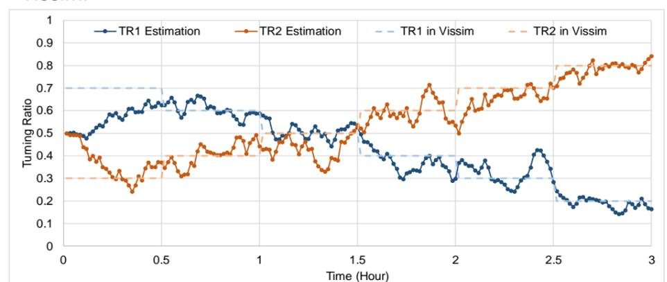
Fig 4: Turning ratio estimation with ECTM based EKF for X-shaped intersection
