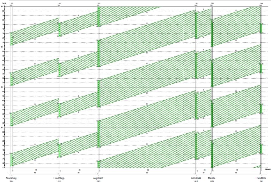
The main goal of this was to define the traffic saturation limits at which the coordination starts failing. At higher traffic volumes, the longer queues of vehicle have been observed in the simulation models. The queues were taking extra time to dissolve, resulting in overall collapse of the coordination. After the analysis, the level of service (LOS) of coordination obtained at various traffic saturation levels have been listed in bar chart on right.
