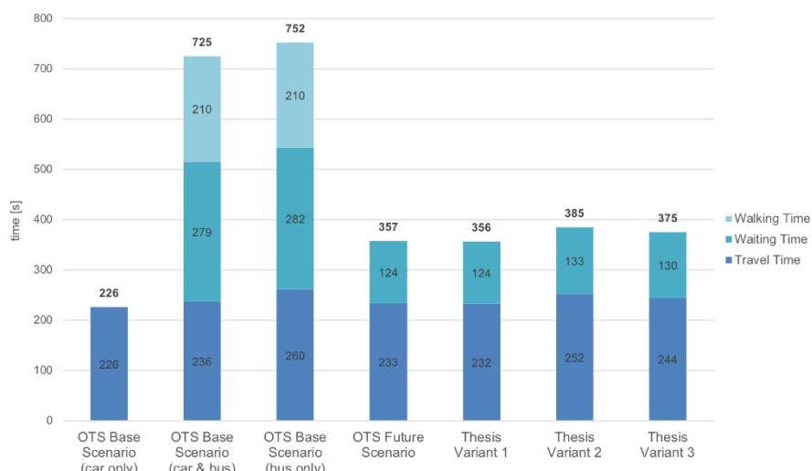
In order to test the approaches, the shuttles were implemented into a microscopic traffic simulation environment with their respective routes. To assess the benefits of the system itself, and distinctly for the developed strategies, a comparative analysis was conducted based on previous results and base scenarios.
